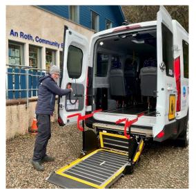
In March, we took delivery of our Maxus all electric minibus. With 10 removable passenger seats, an underfloor wheelchair lift, the vehicle can carry either 10 passengers, or 7 passengers and 1 wheelchair passenger or 4 passengers and 2 wheelchairs. It is really so flexible and well suited for our needs. Alongside the eVito, it is based at Ulva Ferry and charges overnight on our own 7kW EV charger.
